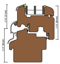
Vertical section of sill in MW88
