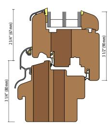
Vertical section of sill in MW88 G2
